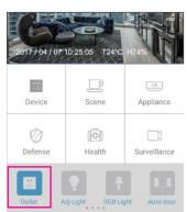
Select Outlet- then click the added device-in line switch, then you can remote control switch and different home appliances, including manual operation switch, auto control, timing control, Scene combination.
