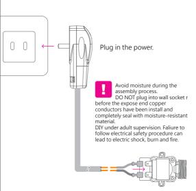
The expose end of the wire to be connected to the terminals on the water valve
