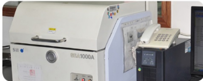
XRF Toxic Heavy Metal Analysis (X-ray Fluorescence)
