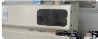
ICP-AES Measure the Concentration of Metal Ions. (Inductively Coupled Plasma with Atomic Emission Spectroscopy)
