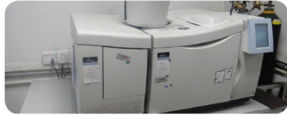
GCMS-QP2010 Organic Material Analysis (Gas Chromatograph Mass Spectrometer)
